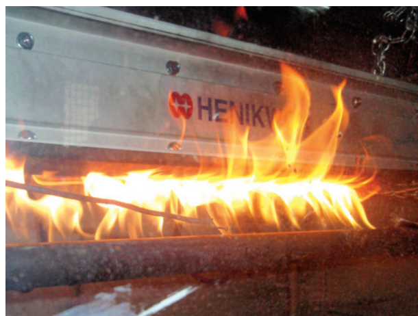
Henikwon Fire-Resistant Busduct System in test chamber burner
