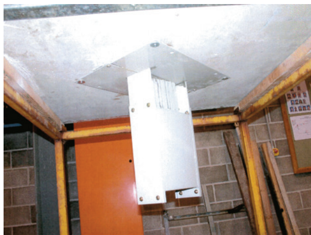
Fire Resistance to building penetration test performed on Henikwon SCM Busduct are BRE, UK
